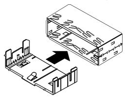
6. Attach the connecting cables to the transceiver unit through the open slot. Slide the transceiver module into the bracket until it clicks into place.
